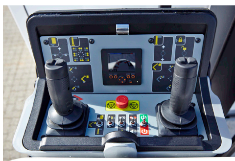
FPC (Full Proportional CANbus controls): Variable outreach (with optional load cell) and up to 4 actions at a time
