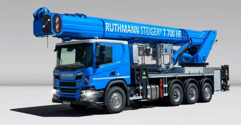
70 m working height with not even 12 m vehicle length! Extremely compact, manouevrable and always operational
